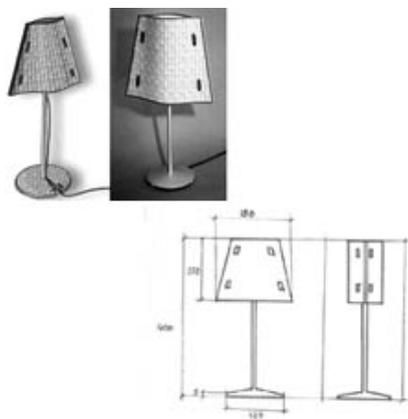
Fig 12. Design process for a lamp in iron and reed.
