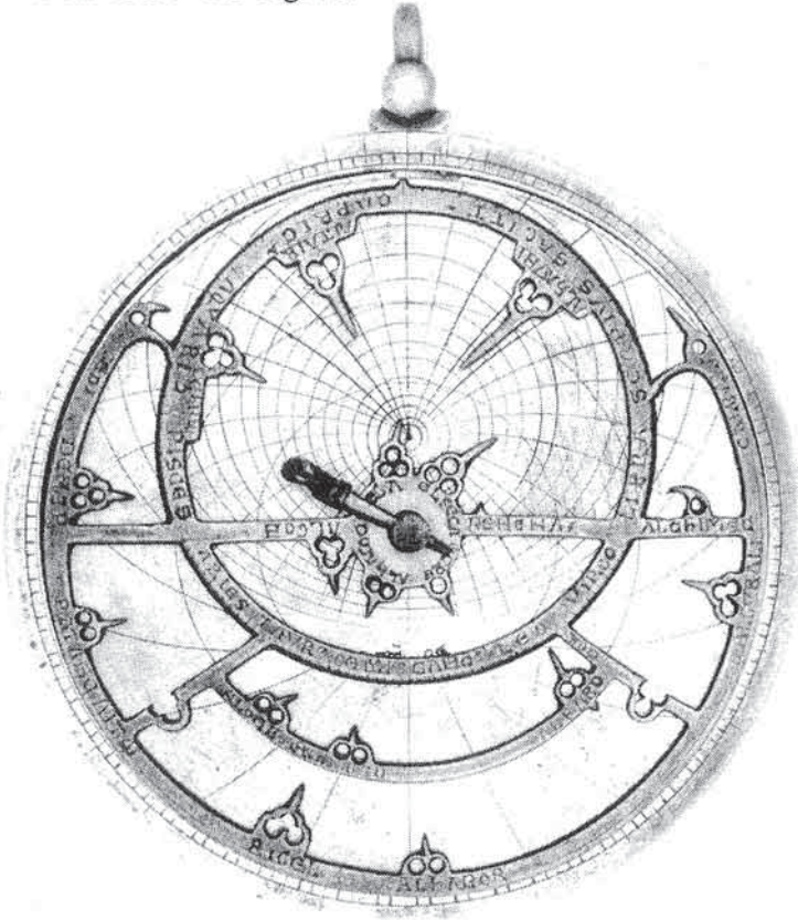
Fig. 13 The front of an astrolabe (#300) with half-quatrefoil insets on the frames supporting the lower equatorial bar, and with star-pointers that bear some resemblance to those on the Spanish astrolabe under discussion (see §3k). [Courtesy of the Museum of the History of Science, Oxford.]
