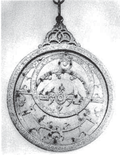
Fig 12a The distinctive rete and distinctive throne on an astrolabe made in Fez in 1319/20 by Muḥammad ibn Qāsīm al-Qurṭubī (#4182). Neither rete nor throne bears any relationship to any other Maghribī astrolabe. Since the maker or his family came from Cordova it seems that we are dealing with a piece that reflects Andalusi influence.
