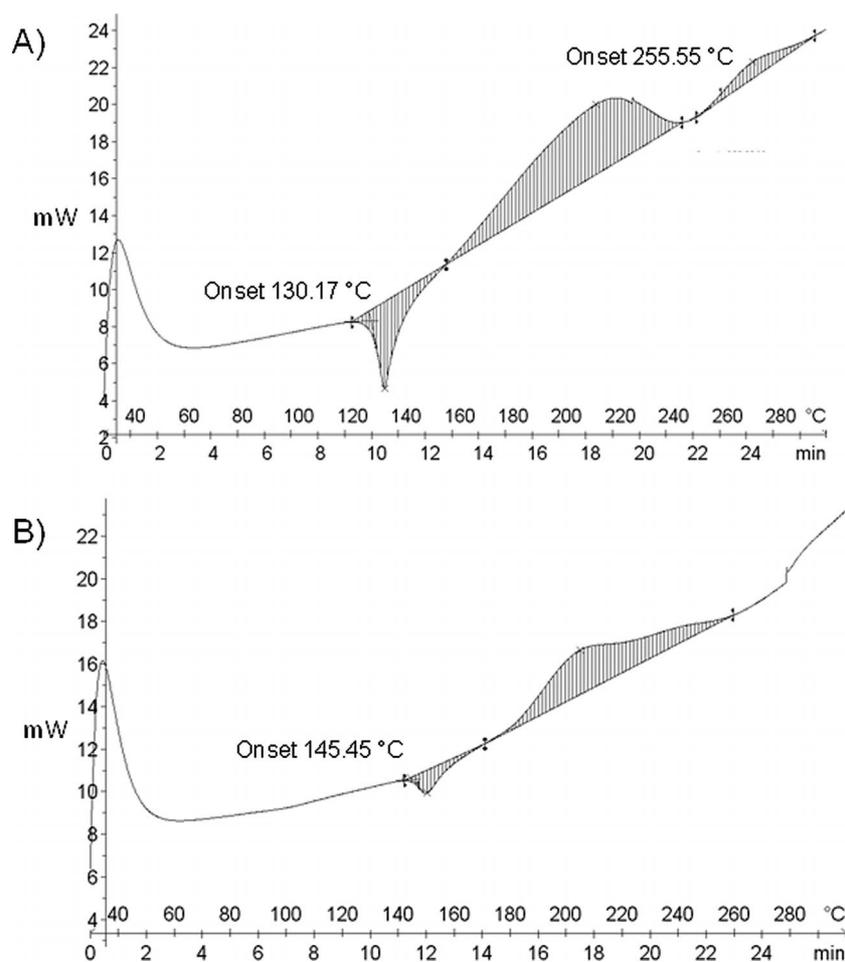
Figure 2. Thermograms showing heat flow vs. temperature and time for DSC experiments with A) OxymaPure, and B) K-Oxyma.
