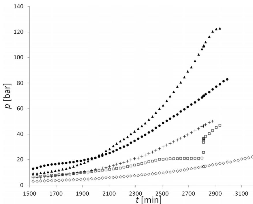
Figure 3. Decomposition profiles of 0.2 M solutions of HOBt (●), HOAt (▲), OxymaPure (□) and K-Oxyma (+) in DMF, together with the solvent (◇) and showing released pressure (bar) as a function of time (min) during ARC experiments.
