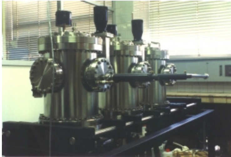
Figure 2.1: Picture of the multichamber HWCVD set-up at University of Barcelona. The three inline UHV chambers were fabricated at the Vacuum Unit of the Scientific-Technical Service of University of Barcelona.
