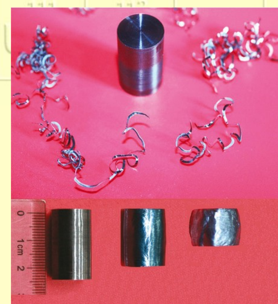
A cylinder of ductile silver sulfide (top) can take a hammering without cracking (bottom, series of hammered cylinders from left).
