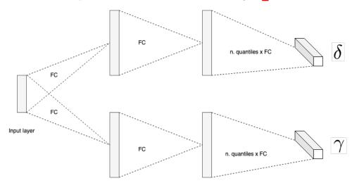
Figure 2: Architectural diagrams of NCDNN. The last layer is composed of as many FC layers as quantiles are calculated simultaneously. FC corresponds to a fully connected layer.
