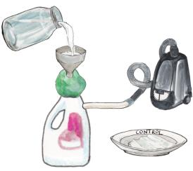
Cover the funnel and the control filter. Turn on the vacuum cleaner and filter the salt solution with the domestic vacuum pump.
