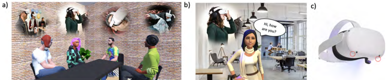
Figure 1. Common auditory scenes in XR. a) Meeting in a virtual room, b) Meeting with an augmented avatar, c) microphone location in the Quest 2 VR Headset.
