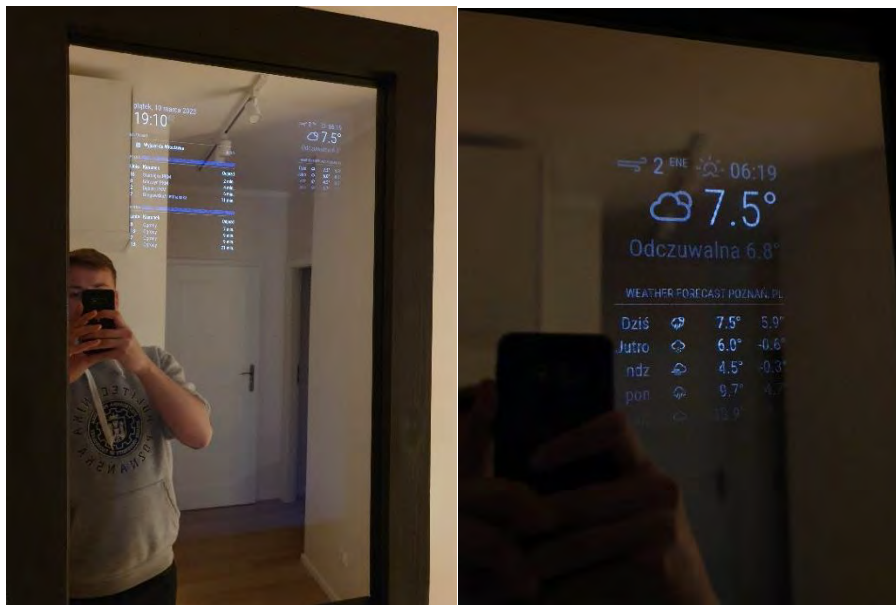
Figure 4. Implementation of the Smart Mirror
