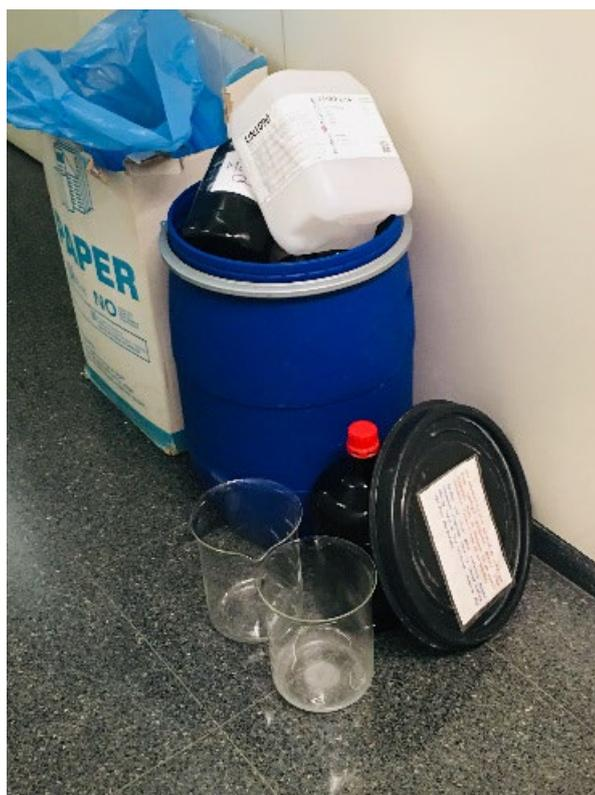
The bins are prepped so that you can open and close them during the waste disposal process touching only the black lid. To this end, **never touch the metal lever-lock**. Doing so can put people in the vicinity of the bins at significant risk of cuts, puncture wounds or impact injuries. The lever-locks are exclusively for use in closing and sealing the bins, an operation that **only authorized technical staff can perform**.
