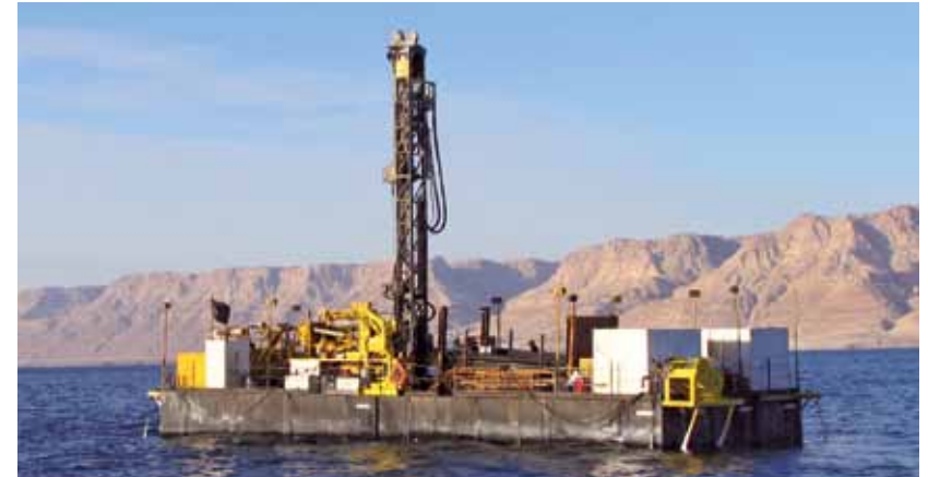
Above An ICDP drill ship at work in the Dead Sea. Both cores of rock and the records of fluid flow and composition are valuable for exploring the subsurface and the minerals and even life-forms it holds.
